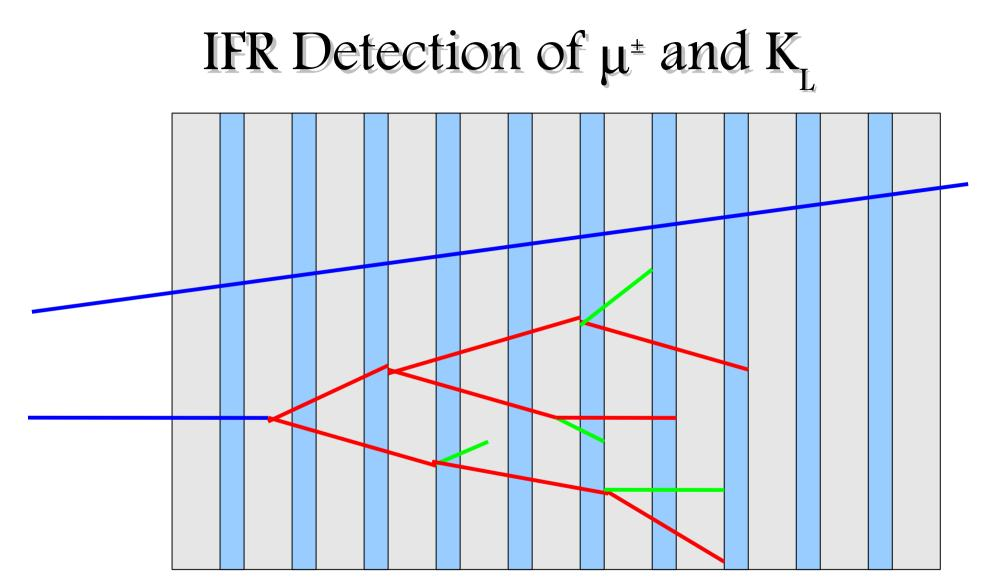
The IFR inserts detector layers into the matter (Fe) to detect the  $K_L$  shower particles. The sufficiently high energy muon passes right though the IFR however, since the interaction length of muons is much longer.
