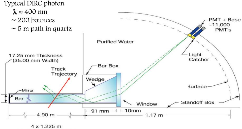
Synthetic Fused Silica Bars glued end-to-end
