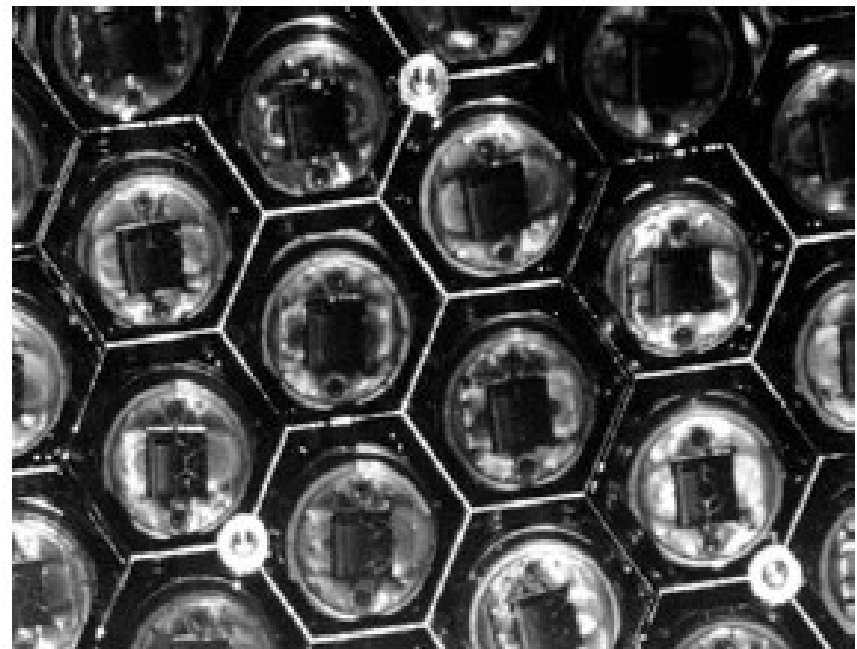
Figure 39. PMTs and rhodium-plated light-catchers in the SOB.
